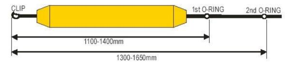
Leash: The length of the leash from the first O-ring to the lanyard webbing shall be a minimum of
